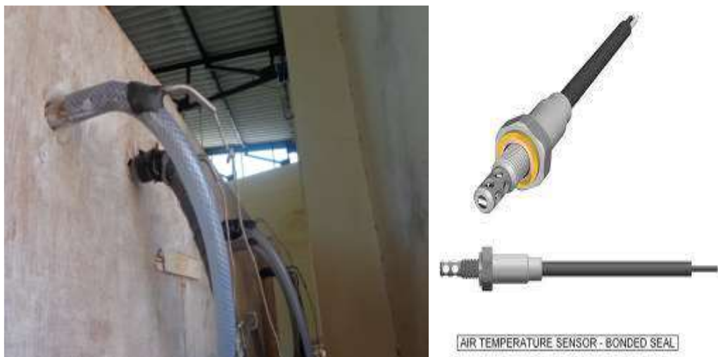
Fig. 5: Air Temperature Transducer
